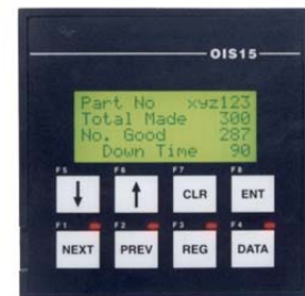
Operator Interface Station
