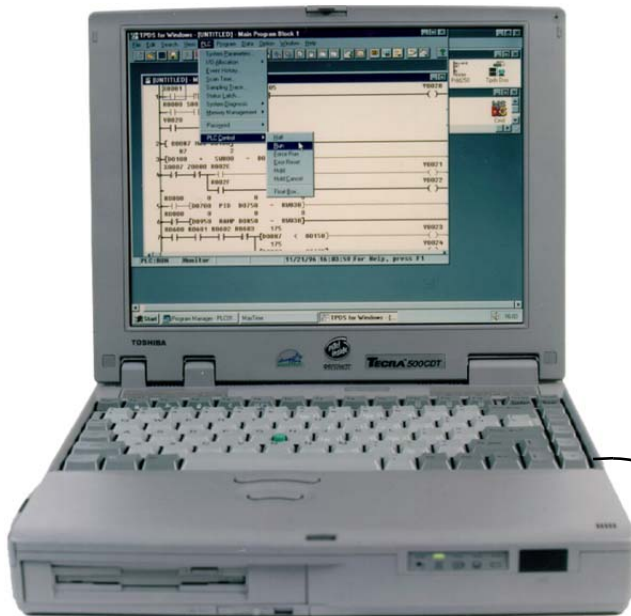
Toshiba Notebook Computer (or Compatible) with T-PDS Windows Programming Software
