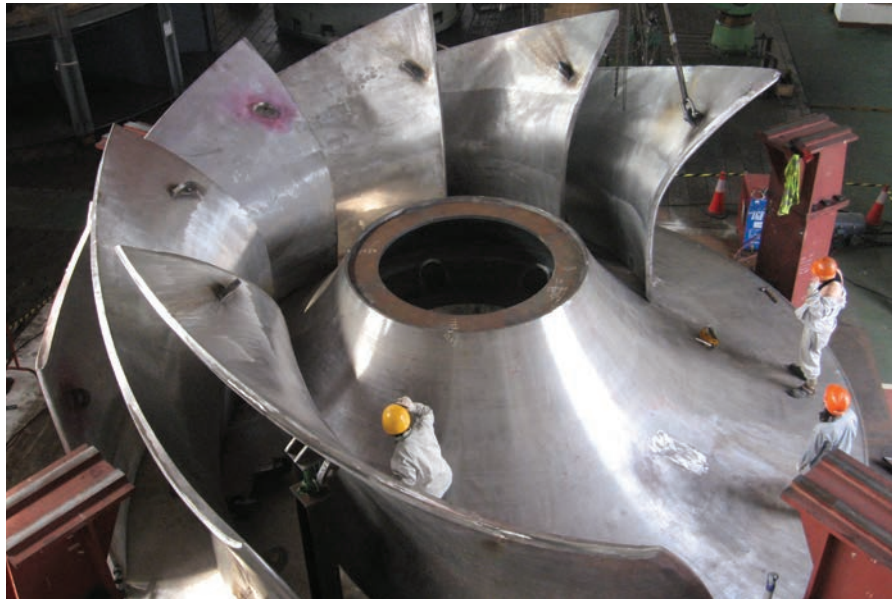
For the new runner, the blade length is longer than a typical nine-blade runner, reducing individual blade load.
