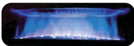
Axial Magnetic Field Interrupter - Arc Dispersion
