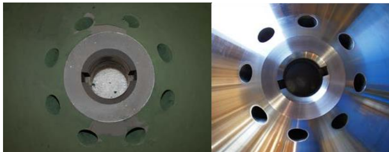
(Left) A CRV Valve Disk with its bore and face nitrided. Note the off-green masking on the remainder of the disk. (Right) The valve disk after polishing and before magnetic particle inspection.
