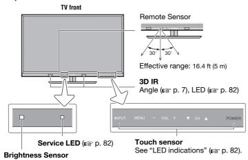
This sensor will detect the ambient light conditions to optimize the backlighting levels ( ${\it les}$  p. 59).
