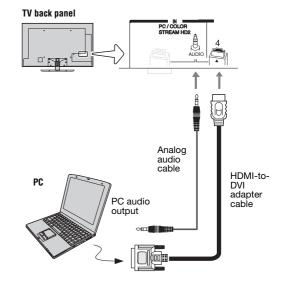
Supported signal formats: VGA, SVGA, XGA, WXGA, SXGA, 480i (60Hz), 480p (60Hz), 720p (60Hz), 1080i (60Hz), and 1080p (24Hz/60Hz). For signal specifications, see p. 86.
