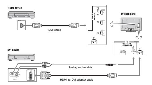
The HDMI input on your TV receives digital audio and uncompressed digital video from an HDMI device, or uncompressed digital video from a DVI (Digital Visual Interface) device.
