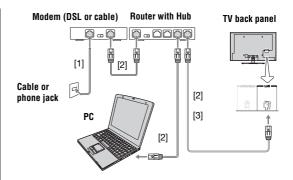
[1] Coaxial or telephone cable (depending on your modem type)
