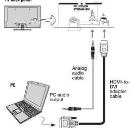
Supported signal formats: VGA, SVGA, XGA, WXGA, SXGA, 480i (60Hz), 480p (60Hz), 720p (60Hz), 1080i (60Hz), and 1080p (24Hz/60Hz). For signal specifications, see p. 84.
