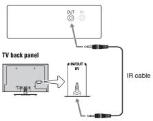
To operate the TV with this connection, point the Toshiba TV remote control toward the front of the IR receiver/repeater control system.
