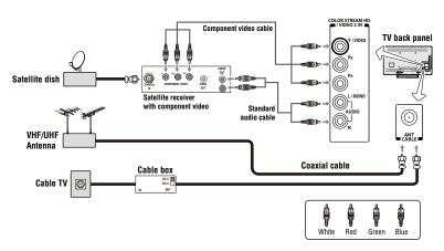
(Sample Illustration) L7400U Series—Connecting to an antenna, satellite receiver, and/or cable TV box
