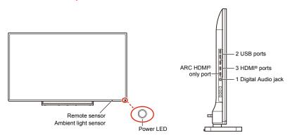
(Sample Illustration) L7400U Series front and side panel controls and connections
